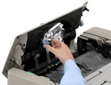
DADF Pickup Roller and Separation Pad Replacement
